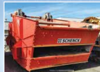
SC3151 3000 x 7300 x 2D Schenck Screen: Double Deck Banana - Complete with Stand, Wet Sump, Drive, Springs, Twin DF601S Exciters. 2 Units Available.
