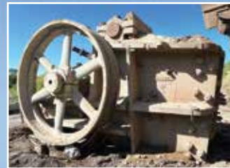
CJ3088 60" x 48" Terex Jacques Jaw Crusher: Double Toggle - Roller Bearing. Condition: Very Good.
