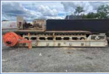
FE3076: 1500 x 6000 RCR Tomlinson Apron Feeder: Complete with Hagglund Drive & Power Pack. Condition : Very Good
