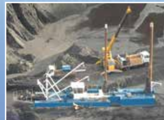
DP3034 10/8 FGH Birdon Marine Dredge: Complete with KTA-19M Cummins Engine, Warman Pump, Rosebud Cutter & Spud Propulsion. Condition: Very Good.
