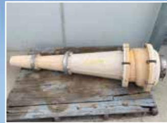
CY3098 250 CVX Weir Warman Cyclone: Cavex – Rubber Lined. Condition: Unused. 4 units available.
