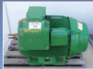
EM4417 90 KW Weg 2 Pole Electric Motor: 2980 RPM – TEFC
