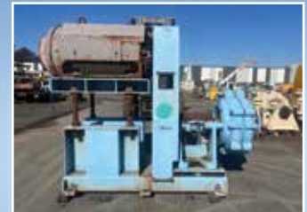
PU3846 10/8 FFM Warman Slurry Pump: Metal Lined - Metal Impeller - Mounted on a F-ZV2 Base with 315 KW Motor. Condition - Very Good
