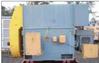
ER3126 1000 KW Toshiba 6 Pole Electric Motor: 985 RPM - CACA
