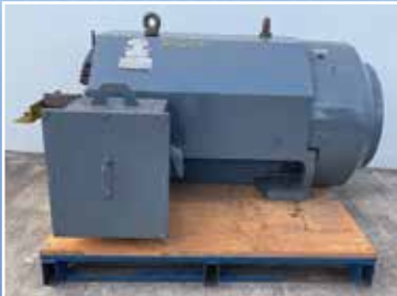
EM4538: 225 KW Teco 6 Pole Electric Motor: 980 RPM 415V – 50HZ Refurbished
