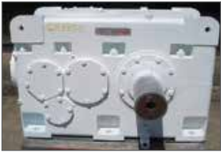
GB3350 990 KW David Brown Gear Box: Model H1-355 – Ratio 5.823 to 1.
