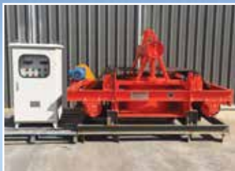
MG3131 800mm M & Q Electro Magnet: Model RCDF-8 – Self Cleaning – Complete with Transformer Rectifier.
