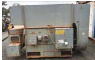
ER3134 1200 KW Toshiba 6 Pole Electric Motor: 985 RPM - 6600 Volts
