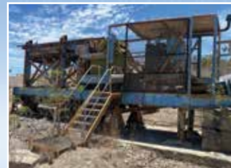
CP3030 36" x 24" Precision Screen Mobile Crushing Plant: Complete with Feed Hopper, Vibrating Grizzly Feeder, Kue Ken Jaw Crusher, Caterpillar Engine & Discharge Conveyor.
