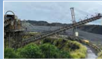
CV3103 750 x 35M M & Q Radial Stacker: Complete with 15KW Drive, One Side Walkway & Powered Wheels. Condition: Good.
