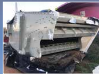
SC3241 3050 x 7320 X2D Joest Screen: Complete with Sub Frame, Drive Motor & Twin JR808 Exciters. Condition: Unused.
