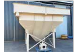
WE3020 4500 x 4500 Linatex Density Bin: 100TPH Sand Washing Bin. Condition: Fully Refurbished.
