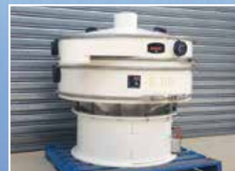
SC3135 48" Kason Screen: Single Deck - Complete with Spacer for Ball Deck & Lid. Condition: Overhauled.
