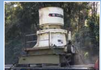
CC3093: J50 Terex Jaques J50 Cone Crusher: Complete with Motor, Lube System & Base Frame.
