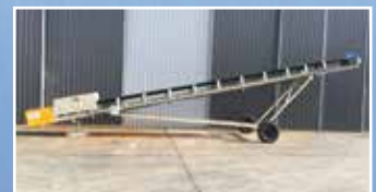
CV3105 - 600 x 12M M & Q Radial Stacker: Complete with 4 KW Drive - DOL Electric Starter - Lanyard Switches.
