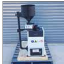
LE3021 100 x 60 M & Q Lab Jaw Crusher: Complete with Hopper, Auto Feeder, Stand & Controller. Condition: New/Unused.
