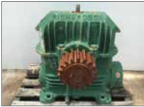
GB3415 12" Radicon Gear Box: Worm & Wheel – 12RHU – Ratio 30.5 to 1.
