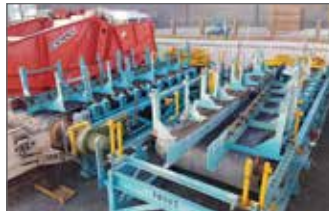
FE3061 1500 x 7500 Bateman Kinhill Belt Feeder: Complete with 30 KW Planetary Drive. Condition: Excellent.
