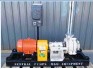
PU3601 3/2 CAH Austral Sand Pump: Metal Lined - Gland Seal - Direct Coupled to 7.5 KW Hi Efficiency Motor & VVVF Drive.
