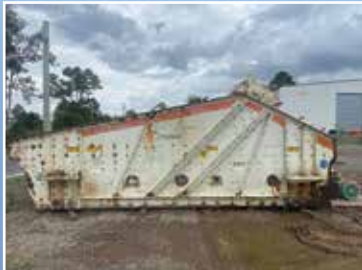
SC3240: 2400 x 6100 x 2D Metso Minerals Screen: Horizontal Dewatering Style – Complete with Motor, Springs & Mounts.
