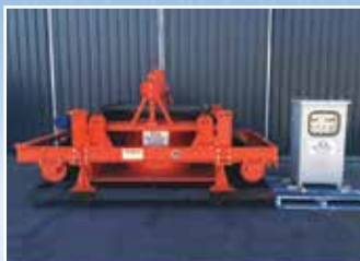
MG3102 1400mm M & Q Electro Magnet: Model RCDF-14 – Self Cleaning – Complete with Tranformer Rectifier.
