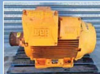
EM4580 90 KW Weg 4 Pole Electric Motor: 1485 RPM – TEFC
