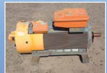
EM4431 400 KW Weg 6 Pole Electric Motor: 989 RPM – TEFC
