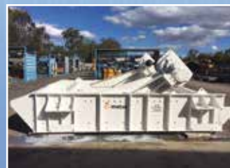
SC3167 3000 x 4800 x 1D Metso / Screenix Screen: Low Head - Dewatering Style - Twin 4-3 Exciters. Condition: As New.
