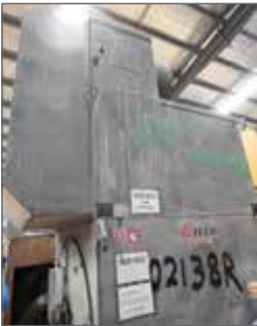
EM4452 1900 KW Teco 12 Pole Electric Motor: 498 RPM – 3300 Volts
