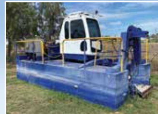
DP3038 4" Vortex Dredge: Single Wire - Auger Cutter. Condition: Very Good.
