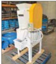
LE3019 8" x 5" Jaques Laboratory Jaw Crusher: Complete with Electric Motor & Stand. Condition: Excellent.
