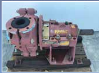
PU3635 4/3 DAH Warman Slurry Pump: Poly Lined - Poly Impeller - Mechanical Seal. Condition: New.
