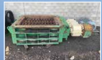
CR3030 600 Abon Sizer: Model 6/160CC - Complete with 132 KW Motor. Condition: Very Good.
