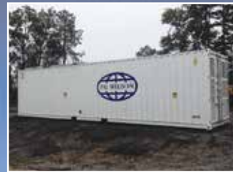
AT3050: 1700 KVA Perkins / FG Wilson Generator Set : Perkins V16 Quad Turbo Engine - 1267 Hours - Complete with Control Panel & Exhaust. 2 Units Available.
