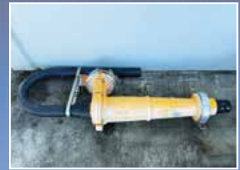
CY3103 100 CVX Weir Cavex Cyclone: Rubber Lined – Complete with Overflow Pipe. Conditon: Unused.
